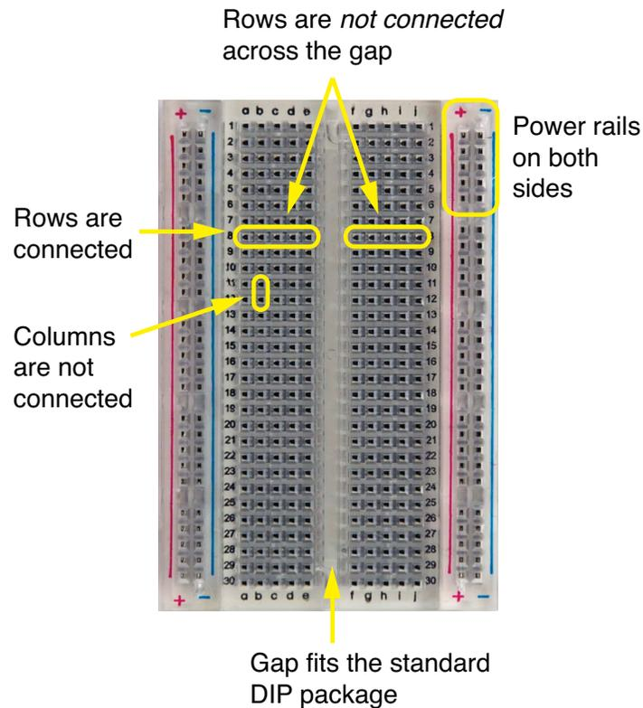
Figure 1: Medium size breadboard with connections highlighted.
