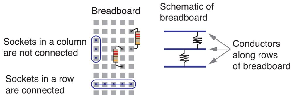
Figure 2: Resistors in series on a breadboard.
