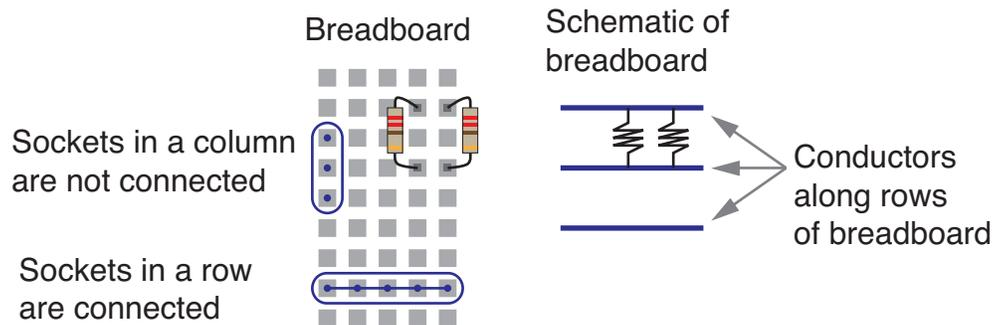
Figure 3: Resistors in parallel on a breadboard.
