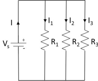
$$R_{eq} = \frac{1}{\frac{1}{R_1} + \frac{1}{R_2} + \frac{1}{R_3}}$$
