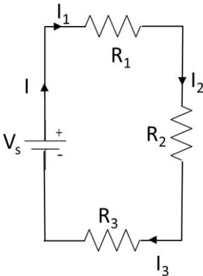
$$R_{eq} = R_1 + R_2 + R_3$$
