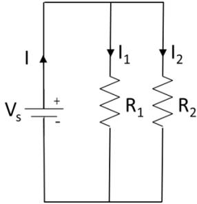
$$R_{eq} = \frac{1}{\frac{1}{R_1} + \frac{1}{R_2}} = \frac{R_1 \cdot R_2}{R_1 + R_2}$$
