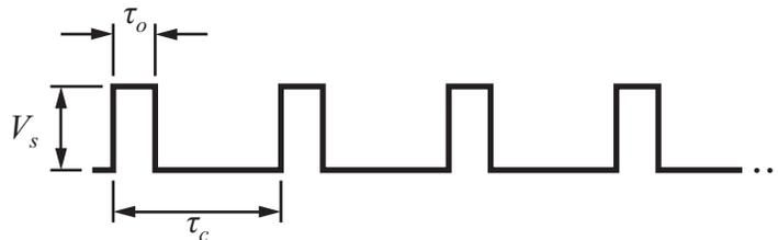
Figure 1: Nomenclature for definition of PWM duty cycle.
